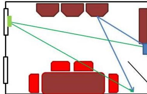
Attention has to be paid to metal panels, metallised glass windows or mirrors, which reflect the majority of the incident power, preventing the signal from passing through. However, some radio power may propagate through small apertures.
