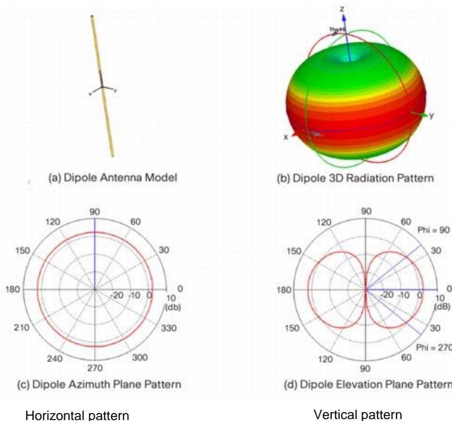
This radiation pattern should be taken into account when designing a WiDup wireless network, in order to ensure that the SH2WBU230N, the SHA4XWLS4, SHE5XWLS4, SHJWD200WExxx, SHJWRE10AExxx, SHJWEM16Axxx in a particular location have coverage on both the vertical and horizontal axes.
