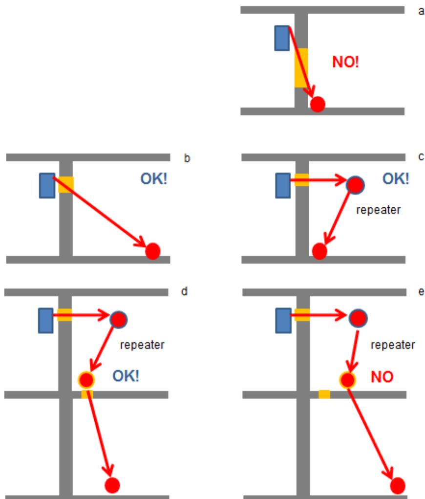
It is also recommended to place a receiver with an internal antenna on the opposite or connecting wall from where the transmitter is placed: this is because near a wall the radio waves might be subject to dispersions and reflections and also because the two antennas should see each other in order to have line-of-sight and the best radio link possible. With reference to the figure below, position a) should be avoided.
