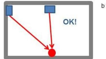
In multi-floor installations, it is advisable to install a SH2WBU230N wireless base unit on each floor in order to have the best radio coverage and to avoid signal attenuation due to heavily reinforced concrete ceilings or floors.
