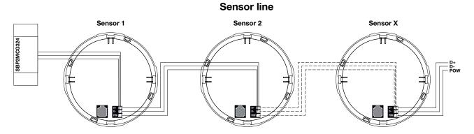
**Note:** The wiring of the sensors must always be made with a 1.5 mm<sup>2</sup> single-core wire, or a stranded wire with ferrules.
