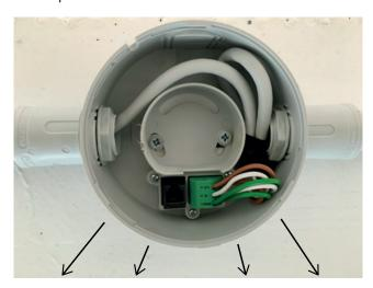
When the sensor is mounted to the base the ultrasonic beams will be send out in this direction.
