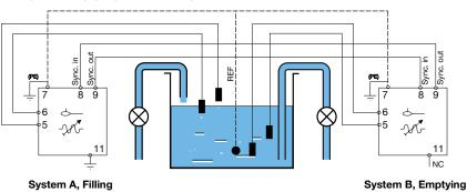
Multilevel application in one tank
