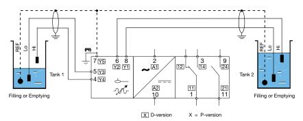
Filling or emptying of up to 2 systems with the same kind of liquid to be measured. Customer can just use one controller for 2 installations.
