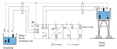
Maximum and minimum control of two systems, a filling system and a emptying system with the same kind of liquid to be measured and one common pump especially in application to transfer from one tank to another tank.
