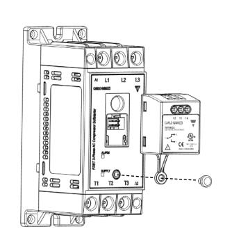
RFPM is a plug-in auxiliary relay module which is provided as an accessory. To install RFPM please proceed as follows:
